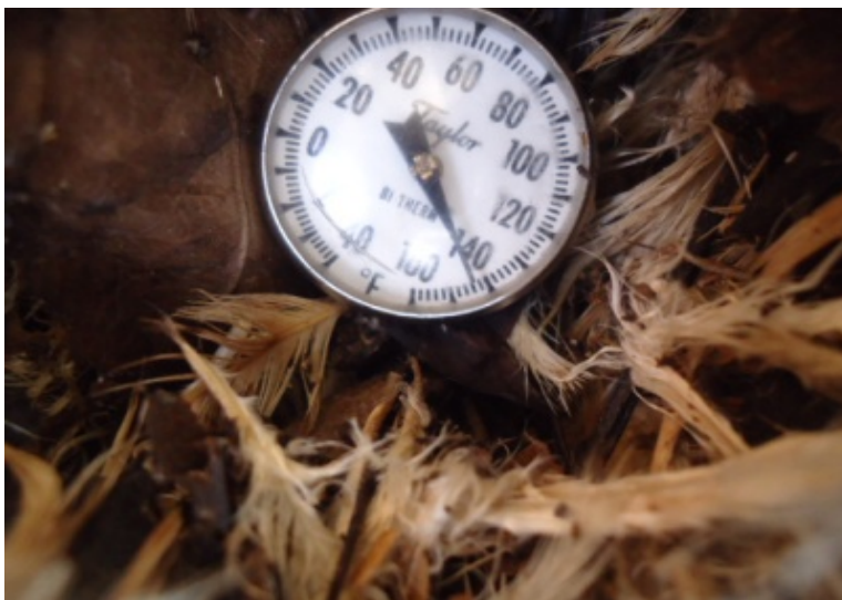
Figure 3. Temperature reached during the composting process (68°C).
